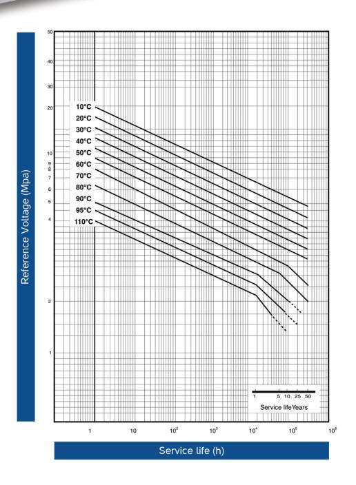
Utilisation Section for Pipes and Fittings of NASSAR According to DINEN Pr 12202
