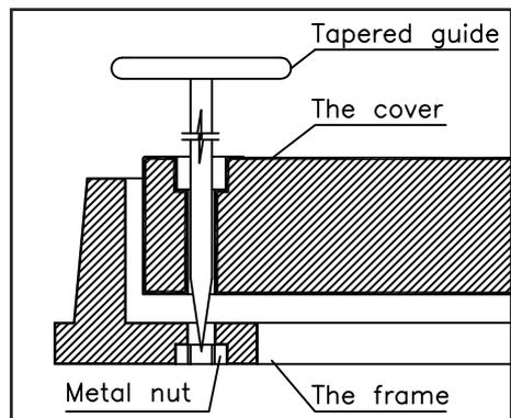
5. To lock the cover to the frame be sure that the lock holes are accurately aligned together and use the screwing T-tool until the screw head is fully flush with the cover top surface.
