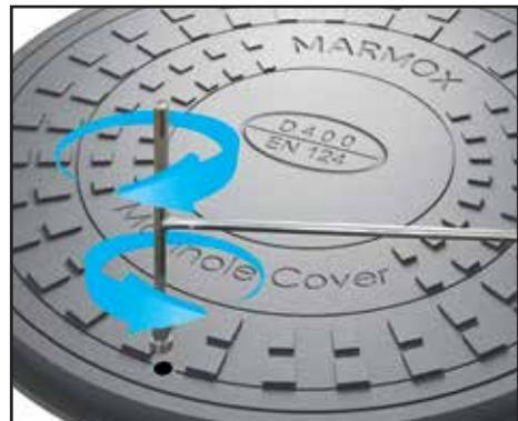
7. To left up the cover use the screw side of the T-tool and screw it in the metal nut fixed at cover bottom and pull up the cover from the frame.
