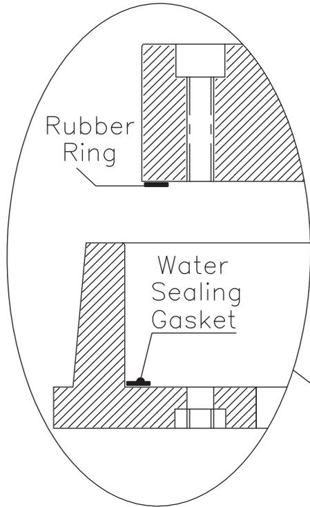
ALL WATERTIGHT MANHOLE COVERS MUST BE INSTALLED BY FIXING SCREWS
